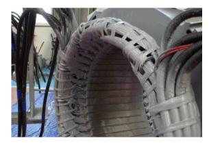
spraying an over coating layer over the impregnated winding, or dipping the stator in a varnish barrel for superior treatments.
